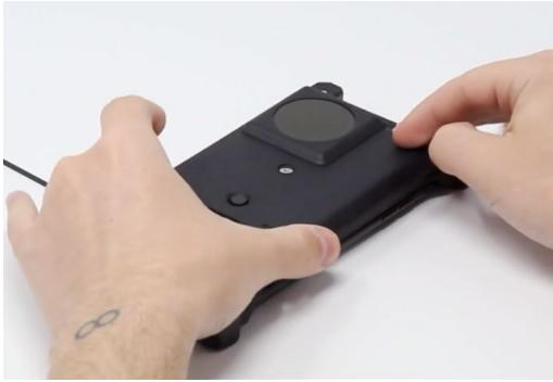
Using the supplied Allen key, tighten the screw until the attractor is properly secured.
